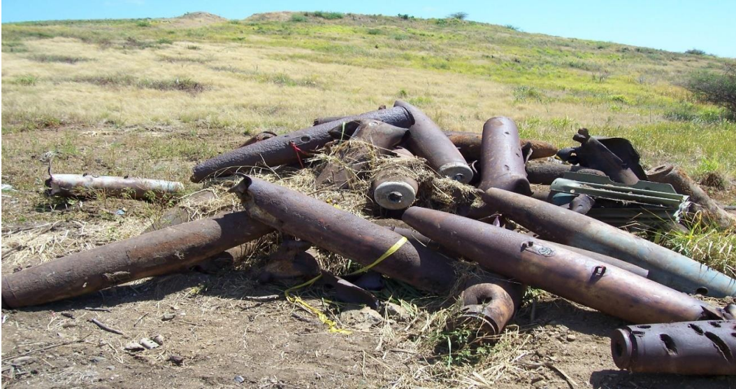
Figure 1.1 Inert MK Series Bombs collected from the surface area of an impact range; Source U.S. Navy
